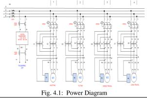
The above power diagram shows the electrical connection of motors. It shows the four motors M1, M2, M3 and M4. Among them M1 motor is for hoisting, M2 motor is for tilting, M3 motor is for cross travelling while M4 motor is used for long travel operation.
